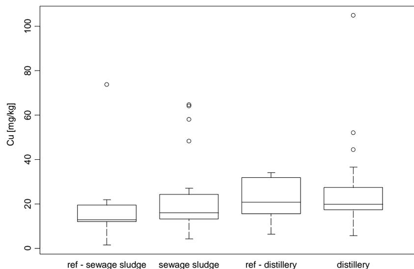
**Figure 4:** Comparison of copper concentrations in fields receiving sewage sludge, distillery by-products and reference fields. Box and whisker plot with the bottom and top of the box being the lower and upper quartile and the band near the middle of the box the median. The ends of the whiskers represent the closest points within the 1.5 interquartile range. Data not included between the whiskers are plotted as a small circle.
