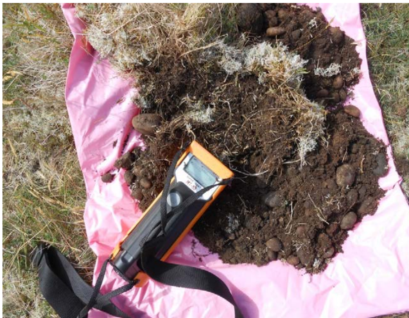
Figure A1-13: Radium 226 identified in spoil by RT-30 2x2 sodium iodide detector
