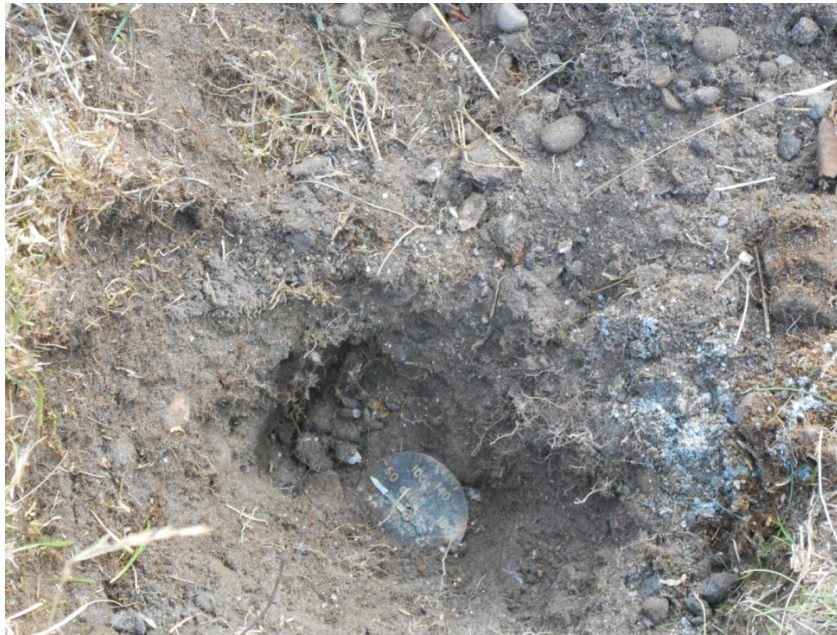
Figure A1-9: Buried dial in excavation pit. Also note blue residue from suspected corroded battery residue (copper sulphate).
