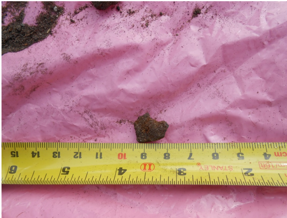
Figure A1-27: Contaminated clinker piece from excavated pit
