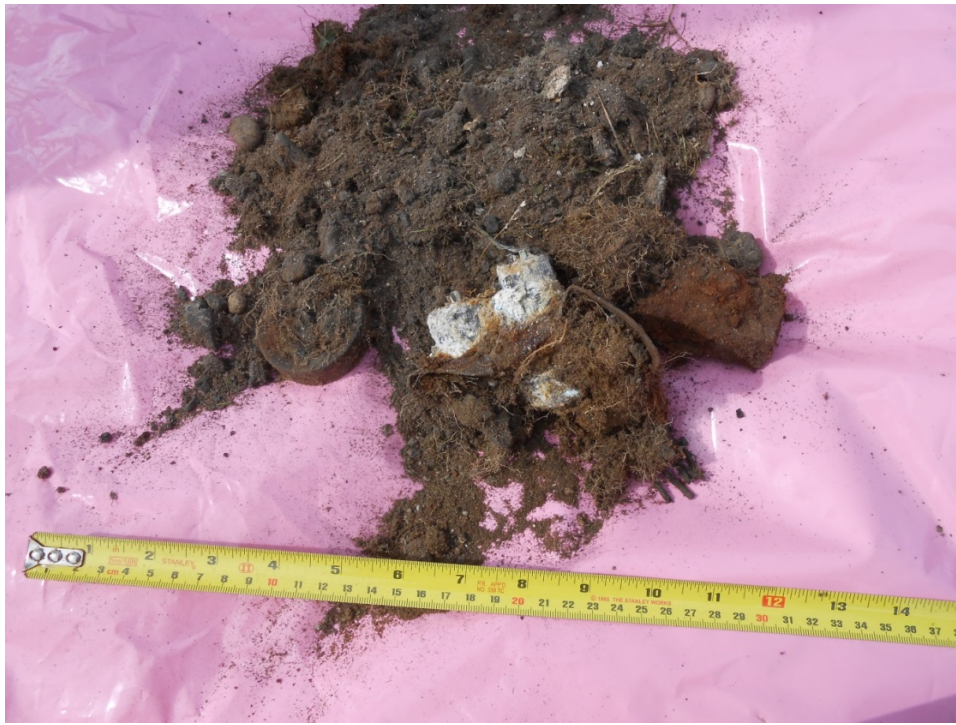
Figure A1-18: Contaminated and other items within spoil from excavated pit
