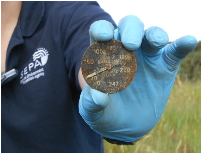
Figure A1-8: Radium luminised dial with needle recovered from excavated area
