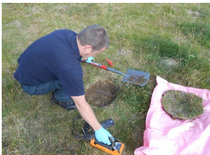
Figure A1-7: Excavation of area showing contamination at approx. 10 cm depth
