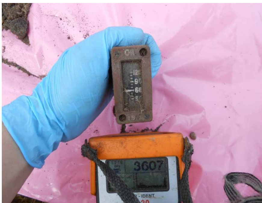
Figure A1-23: Contaminated item recovered from excavated pit (side 2) with RT-30 elevated count
