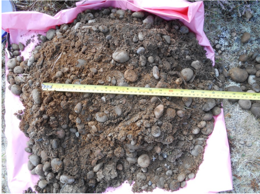
Figure A1-10: Spoil with elevated count rate and no point source
