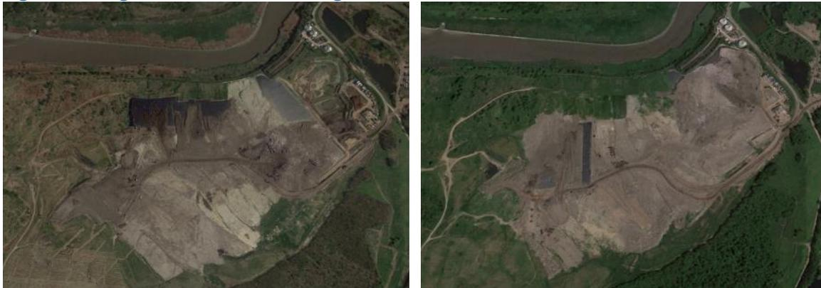
A simple method of measuring change between two data sets is to subtract one from the other, resulting in a separate data layer which details the strength of the change between the two original data layers. The image on the right in Figure 38 is subtracted from the left. Where the pixel values are the same the resulting value is zero (displayed in white) changes produce both positive and negative values with stronger change showing stronger colours.
