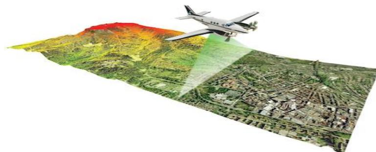
As illustrated schematically in figure 21, a laser pulse is transmitted to the ground target area in a scanning pattern and the pulse is reflected and returned to the receiver where it is measured. The receiver measures the travel time of the pulse and the distance travelled by the pulse is determined by solving the equation (Jaboyedoff et al 2012):
