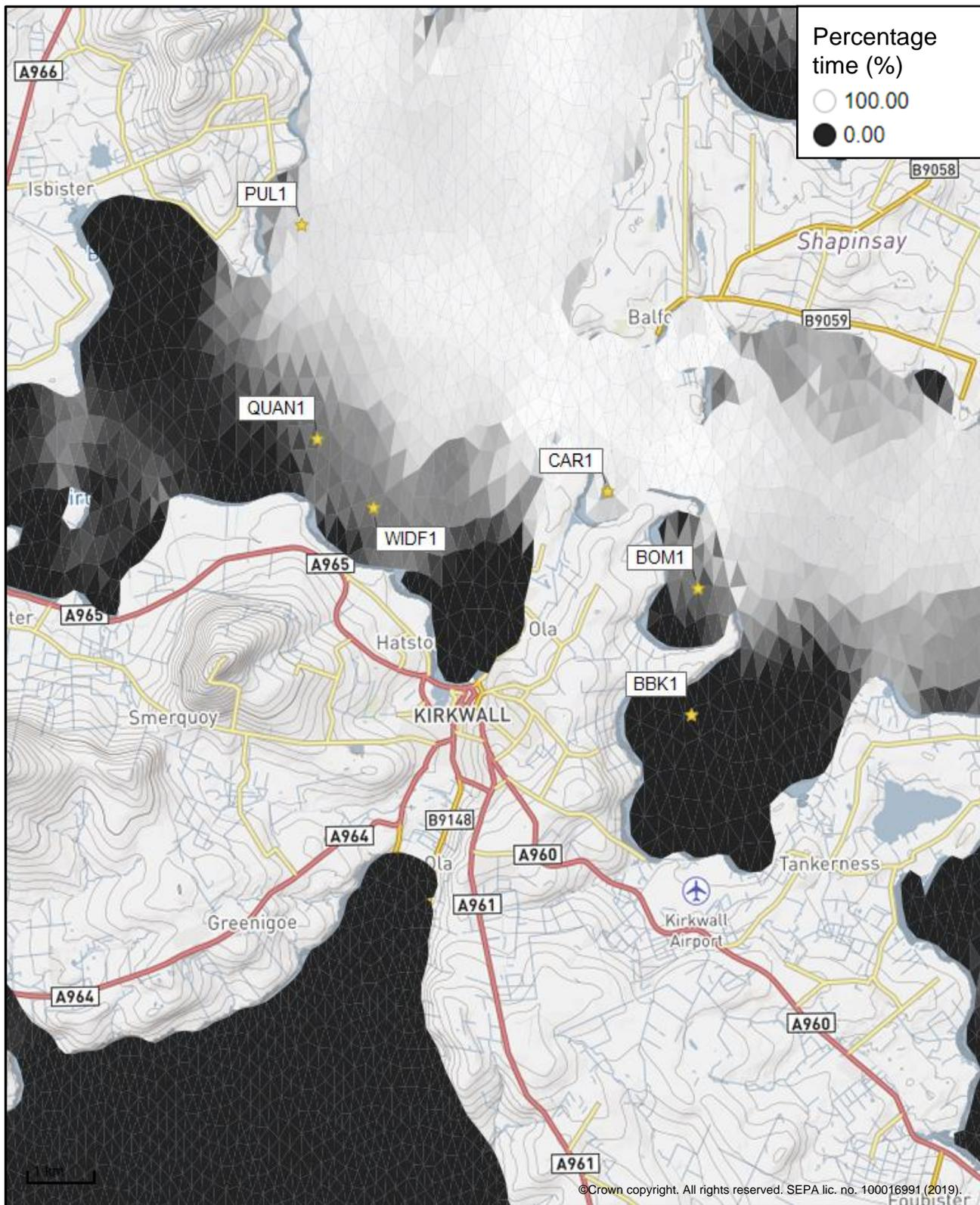
Figure 3: Modelled percentage of time the water flow speed is above 0.095 m/s in the sea area surrounding the proposed site (Quanterness (QUAN1)).
